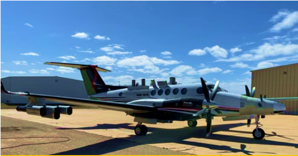
The new University of Wyoming King Air configured with test shapes as part of certification test flights.
